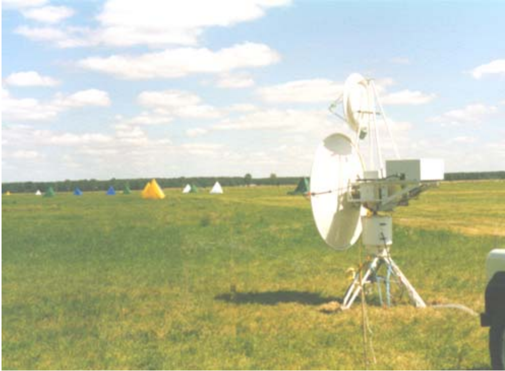
Fig 6. Radar setup with the transmitting dish antenna. The receiving dish antenna on top is tuned to the first harmonic. Both antennae are rotated every 3 seconds by a synchronous motor .
