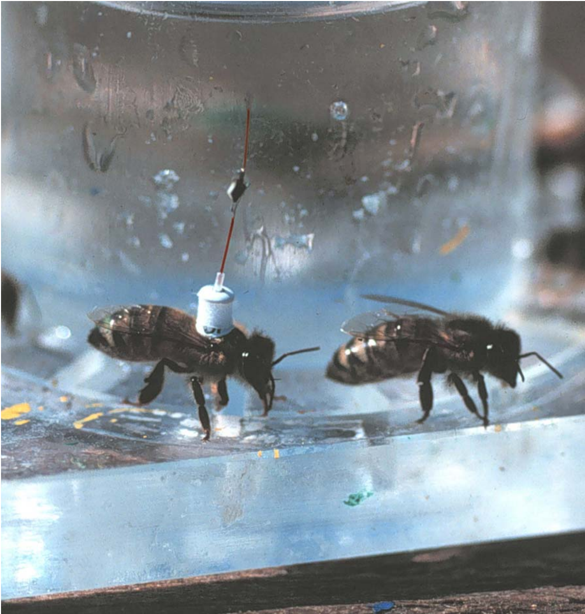
Fig 5. Tiny radar transponders attached to the honeybees' backs allowed us to track the insects' flight paths while foraging. The dipole-based transponder reflects the radar transmitter frequency's first harmonic, which can be easily discriminated from typical background radar reflections.
